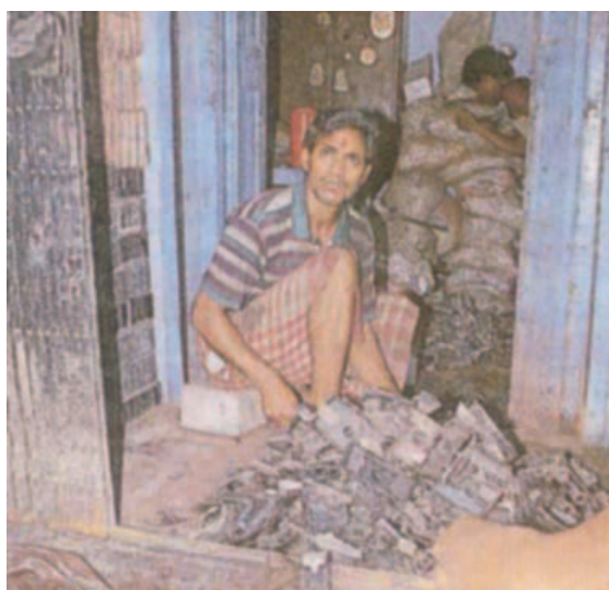
An occupational health hazard - Lead battery plates being broken down by hand
