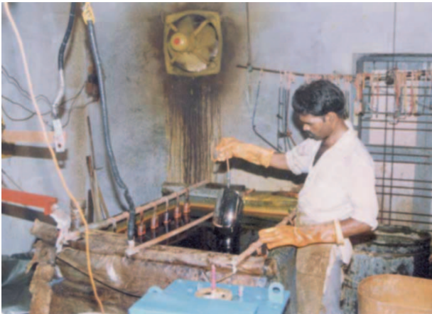
Small scale enterprise - zinc cyanide electroplating unit
