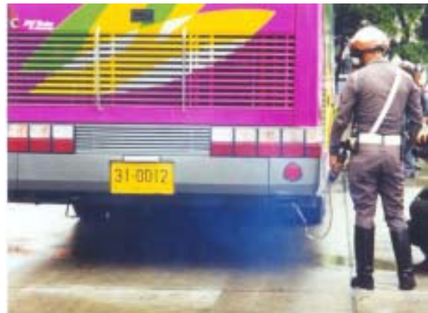
Figure 9.3 Black Smoke Inspection
