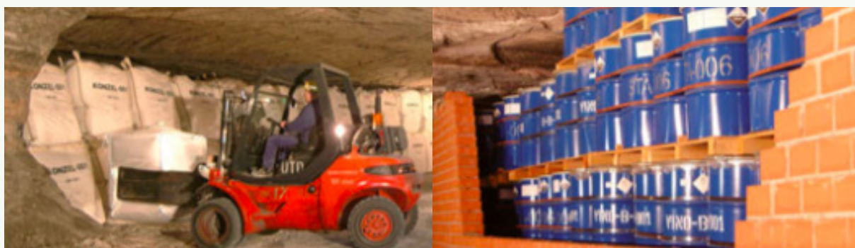
Placement of bags and drum containers in the Herfra Neurode salt mine 53
