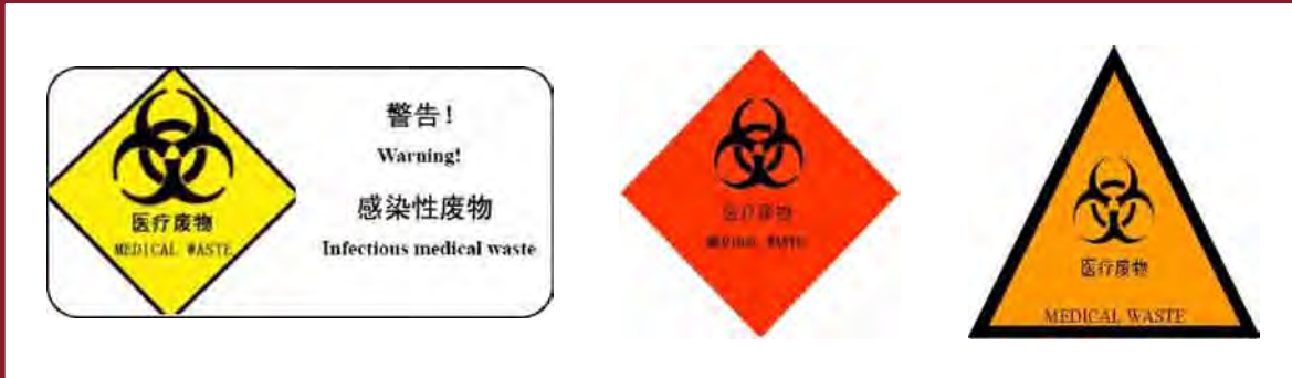
left: Symbol for packaging bags and containers of healthcare waste center: Symbol for healthcare waste transportation vehicle right: Symbol for temporary storage site of healthcare waste
