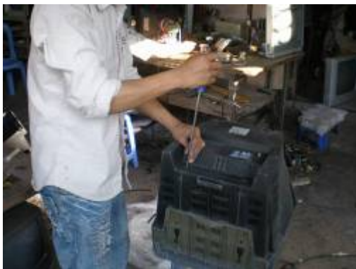
Picture 1: the repairer is screwing out to take usable parts
