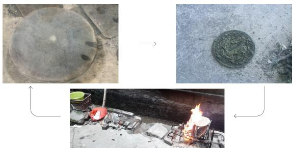
Burning to remove plastics on filter mesh
