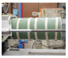
(b) Insulation layer is installed on extruder
